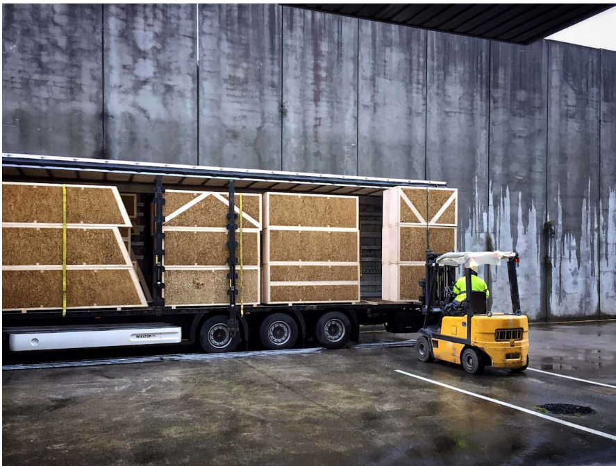
Fast-growing plants have been used structurally for millennia. Contemporary experimentation with such materials in the global north is developing ways of slotting them into an intransigent industry geared towards mineral materials. Below, EcoCocon, a manufacturer of straw and timber construction panels, prepare a shipment Credit:EcoCocon®
